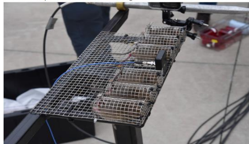
Mice in prone position placed in metal mesh platforms allowing unimpeded blast wave travel
